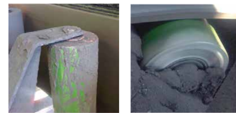
Ideal for wet and dirty operating conditions on generally short conveyors and loading zones.
